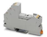
RIF-1... relay base, for miniature power relay with 1 or 2 PDTs or solid-state relays of the same design, push-in connection, plug-in option for input/suppressor modules, for mounting on NS 35/7,5
