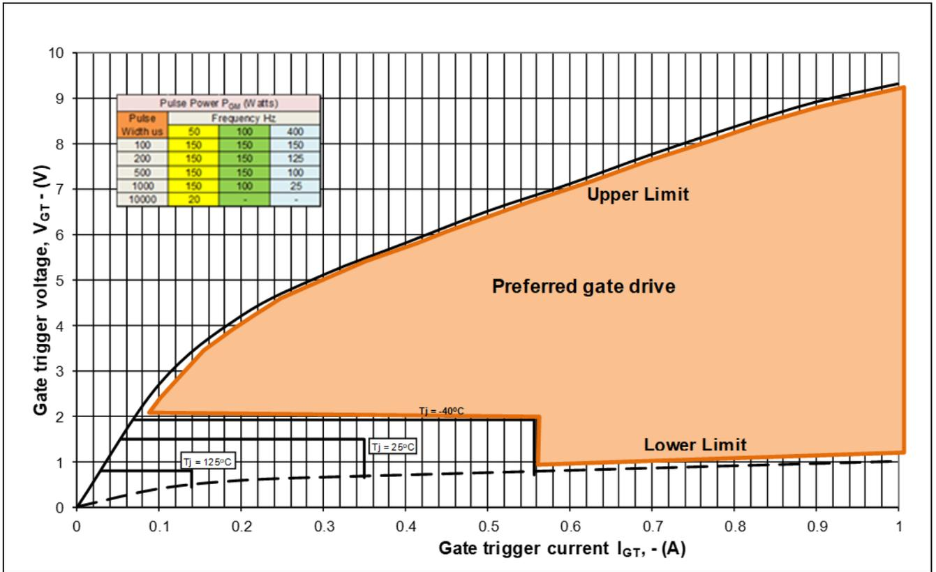
Fig. 14 Gate characteristics
