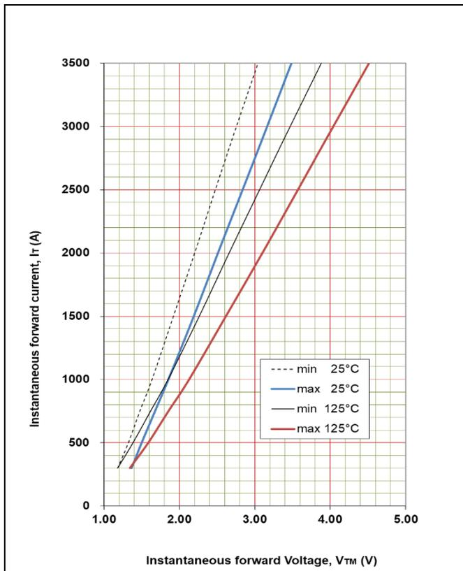
Fig. 2 Maximum & minimum on state characteristics
