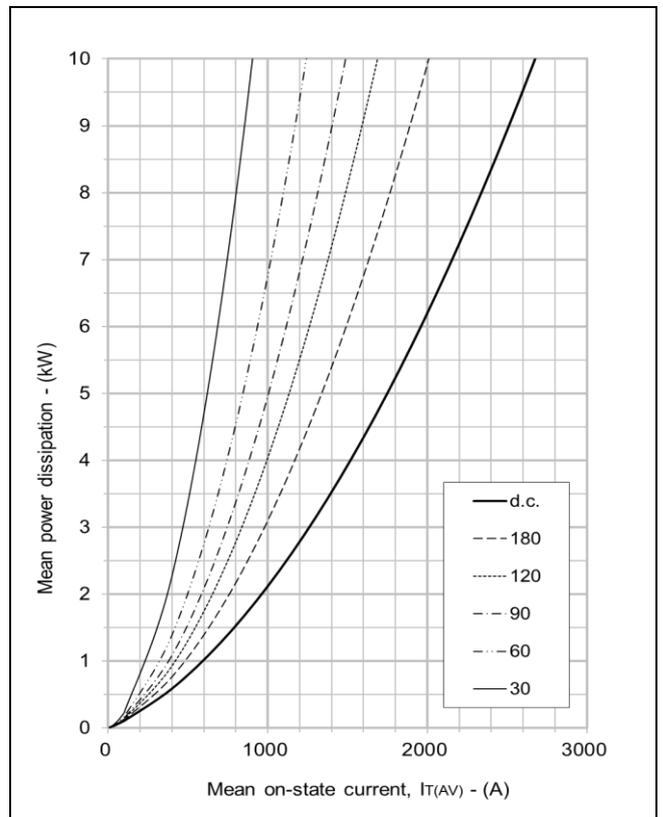
Fig. 6 On-state power dissipation - rectangular wave
