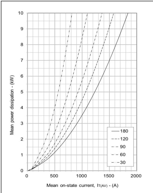
Fig. 3 On-state power dissipation - sine wave
