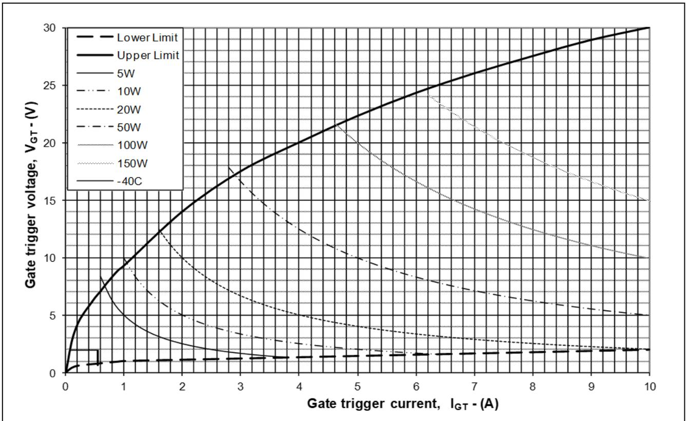
Fig. 15 Gate characteristics
