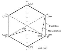
Sample: G5Q-1A-EL-HA-VH Number of Relays: 5 pcs Test conditions: Measure the value of contact malfunction happening by applying 3 axes with 6 direction 3 times each.
