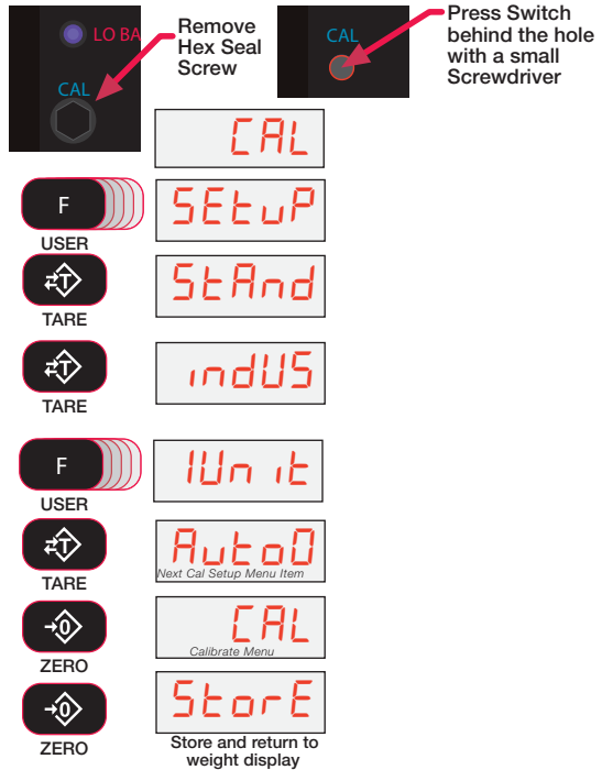
Figure 5-9. Weight Standard Setup
