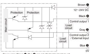
Power wires (Brown 1. Blue 3) are not attached to Handset unit, both on cable and connector type.
