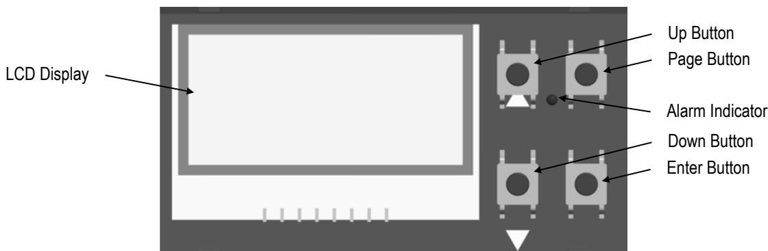
Figure 33: Control Panel for the Comm Box (DIN)
